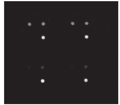
Q-View™ Imager generated image demonstrating typical sample results and reproducibility (samples shown were run in duplicates in each row). Samples can be run in duplicate or singlet allowing 45 to 90 unique samples to be run simultaneously on the same plate.
